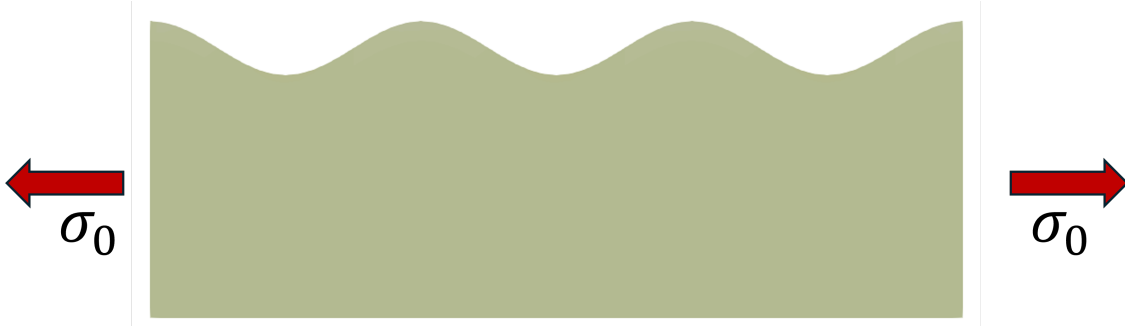
Figure 1.1: Schematic of a sinusoidally perturbed surface where the underlying substrate is subjected to in-plane stress of \sigma_0 . The perturbation of the surface is exaggerated for clarity. The evolution of the surface via surface diffusion was analytically solved for by Asaro and Tiller [1] and Grinfeld [2], which provides a useful benchmark for testing the finite element formulation and implementation.
